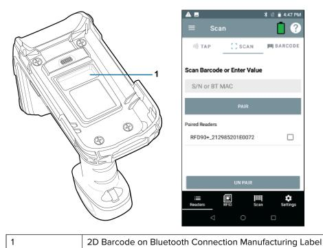
To connect via NFC, align the NFC area behind the sled handle with the NFC area on the back of the mobile computer to pair.
