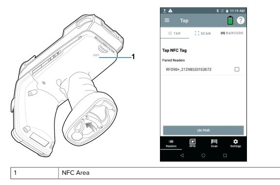
Once the mobile computer has paired with the sled, it recognizes the device going forward and automatically connects using the 123RFID Mobile.
