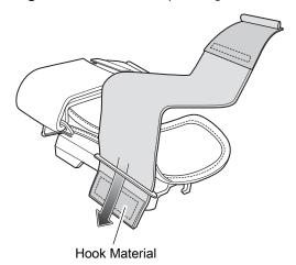
Figure 115 Feed Strap through Rear Slots
