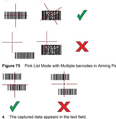
Figure 75 Pick List Mode with Multiple barcodes in Aiming Pattern
