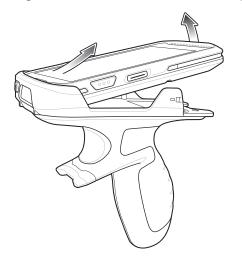
Figure 106 Remove Device from Trigger Handle
