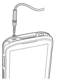
2. Connect the 3.5 mm connector plug of the headset into the 3.5 mm Audio Adapter.
