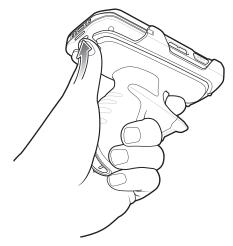
2. Slide the device away from the front of the Trigger Handle.
