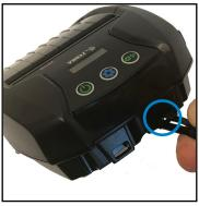
Clip one end of the shoulder strap to the post (circled) on the front side of the printer.
