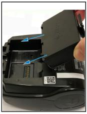
4. Rock the battery into the compartment as shown until it locks in place.
