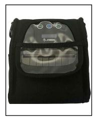
Turn the case around to access the LCD display and user controls which are visible through the plastic window. The bottom half of the plastic window can be lifted to access the paper path.
