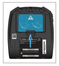
3. Rotate the pack away from the battery well. Lift the battery up and out of the printer.
