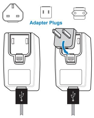
Install the adapter plug into the Power Supply by hooking the top edge into the adapter's receptacle cavity and rotating it until it snaps into place.
