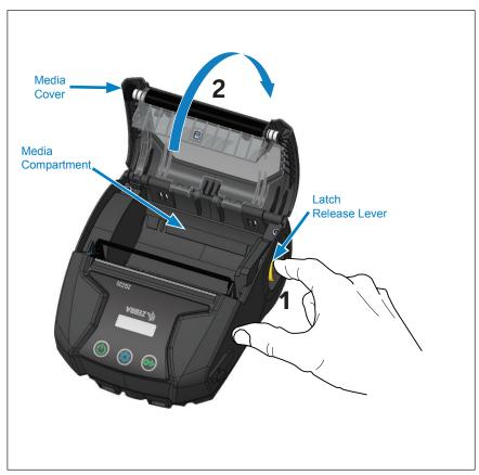
Figure 3 • Opening the Printer
