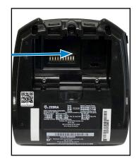
3. Insert the battery into the printer as shown. (It is not possible to insert the pack in the incorrect orientation.)
